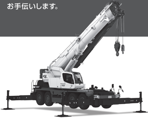
ROUGH TERRAIN CRANE [CREVO]
