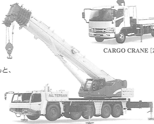
ALL TERRAIN CRANE
